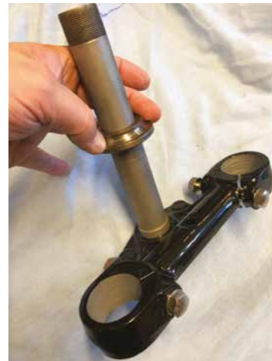
Morgan refitted the original bearing track, having checked it for absence of damage. Note that the areas of yoke masked off are now in bare shot-blast finish. Judicious application of grease will make future dismantling a breeze. Now is the time for those stainless fasteners!
