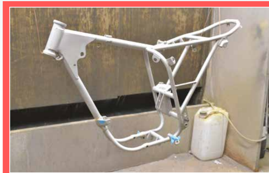
The freshly blasted kit is hung from a conveyor which carries it through the next stages
