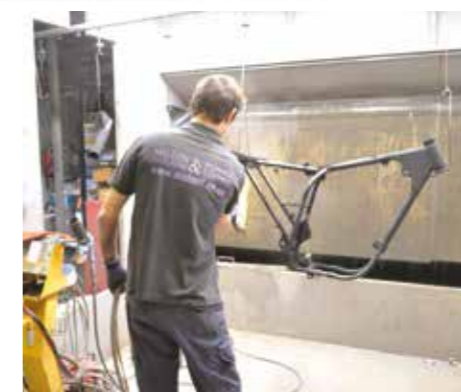
The frame gets its top coat applied
