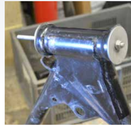
Part of the preparation involves sealing off those areas where blasting and coating would not be helpful...
