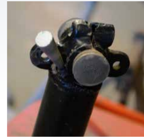
The sealing-off business is considerably important. Observe the sundry bungs used on this BSA fork slider
